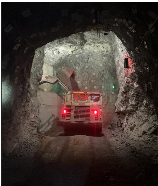
Figure 15 - AD1140 Truck loading bay at bottom of ore pass
